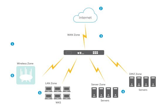
• By leveraging expansive network interface density and a segmented topology, the firewall should be able to segment multiple network areas into a single security appliance delivery.
